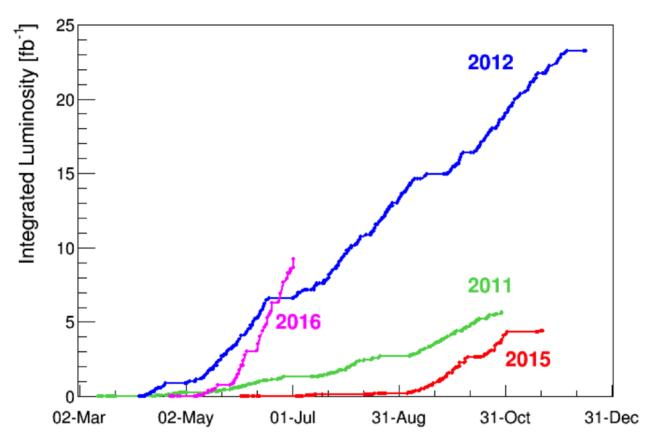
This graph shows the integrated luminosity delivered by the LHC to the ATLAS and CMS experiments in 2011, 2012, 2015 and 2016. The integrated luminosity indicates the amount of data delivered to the experiments and is measured in inverse femtobarns. One inverse femtobarn corresponds to around **80** million million collisions.
