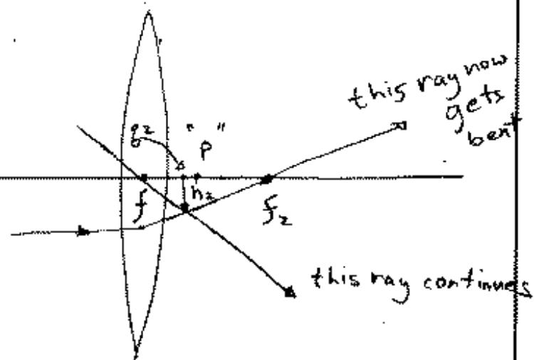
" $p$ " was the position of the 1st image ( $h'$ ), but now is the position of a virtual object of height  $h'$ , at a distance of " $p$ " from the center of a second lens. Let's work an example:
