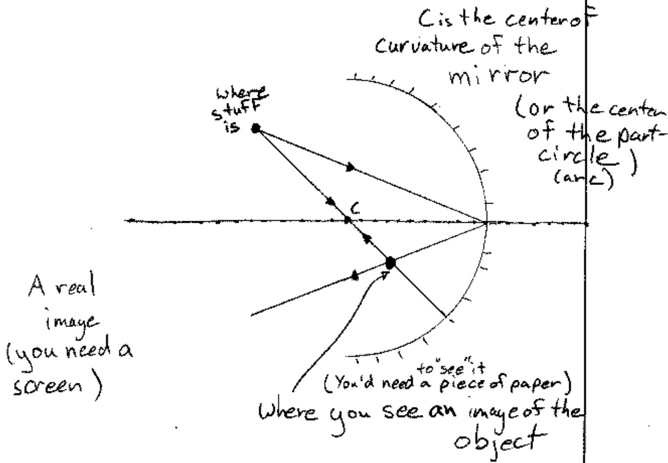
the ray that is reflected back on itself will, or will try to go through the center of curvature.
