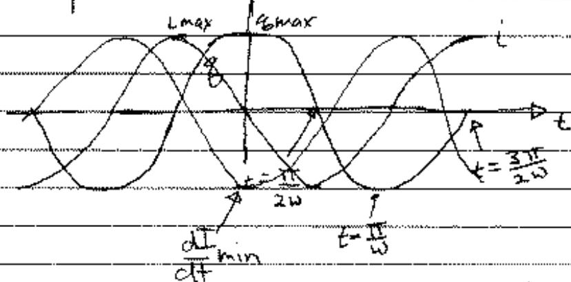
voltage and current are out of phase  $i_{\max}$  before  $q_{\max}$
