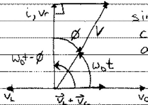
since we define the current to have an angle  $\omega_0 t - \phi$  we have to define how we calculate it
