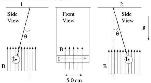
If B = 0.01T, and the mass of the wire is 40 grams, what is the angle at which the pendulum hangs when 1.0 A flows in the wire? (10 pts) (Treat the support wires as being massless)
