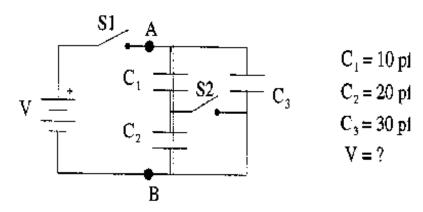
a) We close only switch S1 and notice that a long time later (at electrostatic equilibrium) the charge on  $C_3 = 7.0pC$ . What is the potential difference of the battery?
