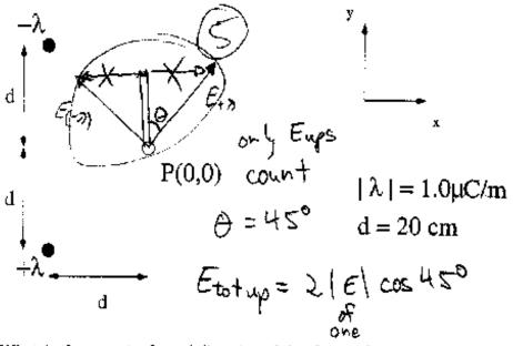
a) What is the magnitude and direction of the electric field at the point P (0,0)?
