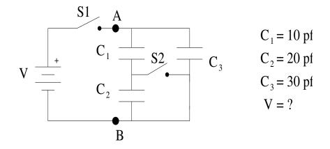
a) We close only switch S1 and notice that a long time later (at electrostatic equilibrium) the charge on  $C_3 = 7.0pC$ . What is the potential difference of the battery?
