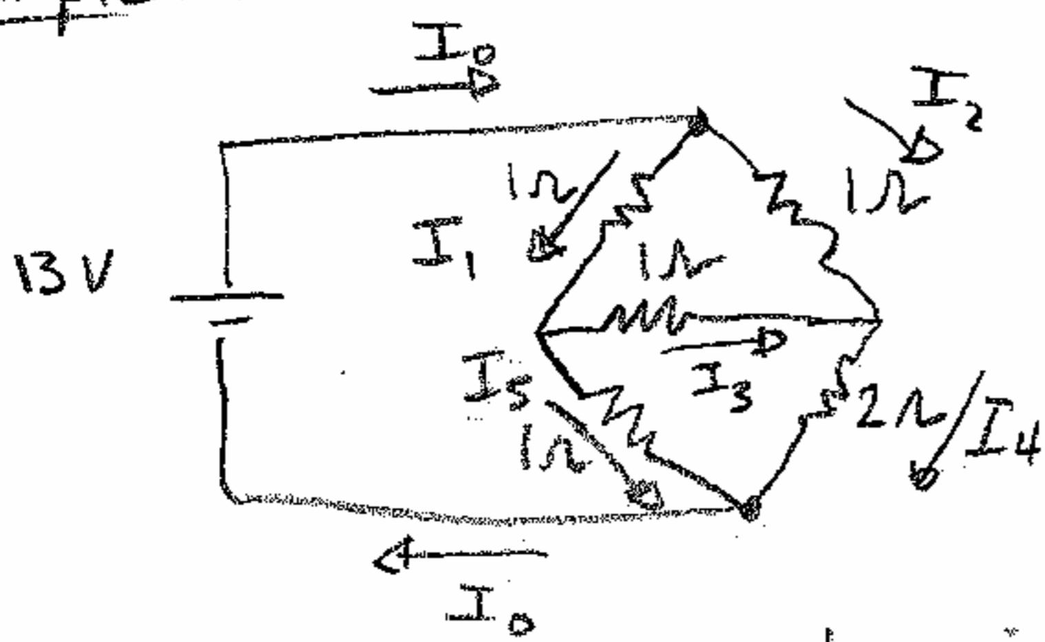
$$\begin{aligned} I_0 &= I_1 + I_2 \\ I_1 &= I_3 + I_5 \\ I_2 &= I_4 - I_3 \\ I_5 + I_4 &= I_0 \end{aligned}$$
