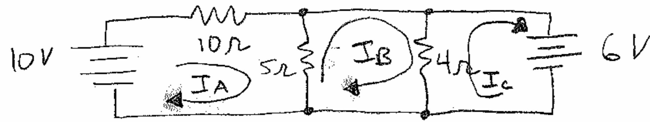
Note: current through  $5\Omega$  is  $I_A - I_B$
