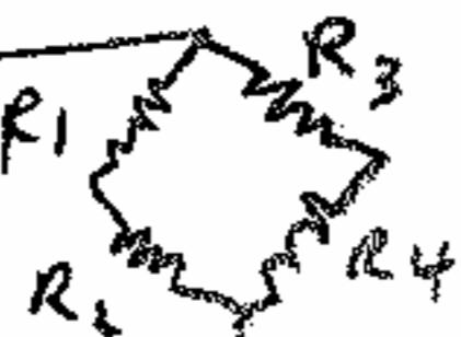
$$\begin{aligned} I_1 &= I_5 & I_1R_1 &= I_2R_3 \\ I_2 &= I_4 & I_1R_2 &= I_2R_4 \end{aligned}$$
