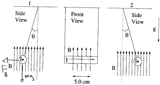
If B = 0.01T, and the mass of the wire is 40 grams, what is the angle at which the pendulum hangs when 1.0 A flows in the wire? (10 pts)
