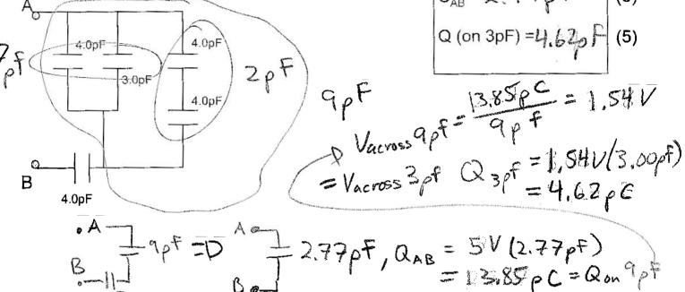
b) Now, the battery is removed, but the charge remains on the capacitors. If an uncharged 5.0 pF capacitor is now hooked up between points A and B, what is the charge on the 3.0 pF capacitor at electrostatic equilibrium?
