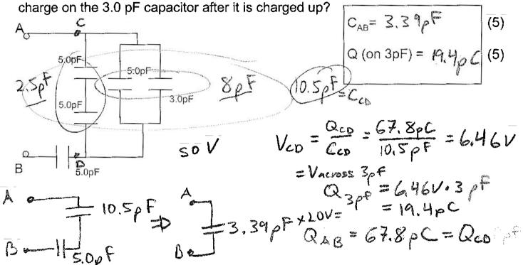
b) Now, the battery is removed, but the charge remains on the capacitors. If an uncharged 6.0 pF capacitor is now hooked up between points A and B, what is the charge on the 3.0 pF capacitor at electrostatic equilibrium?
