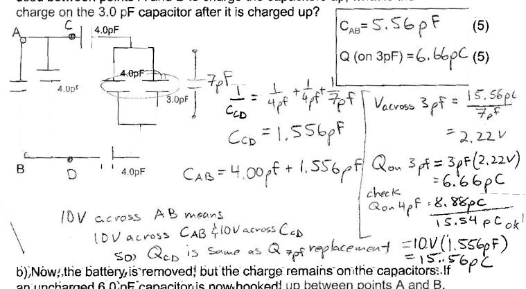
an uncharged 6.0 ph capacitor is now hooked up between points A and B, what is the charge on the 3.0 pF capacitor at electrostatic equilibrium?
