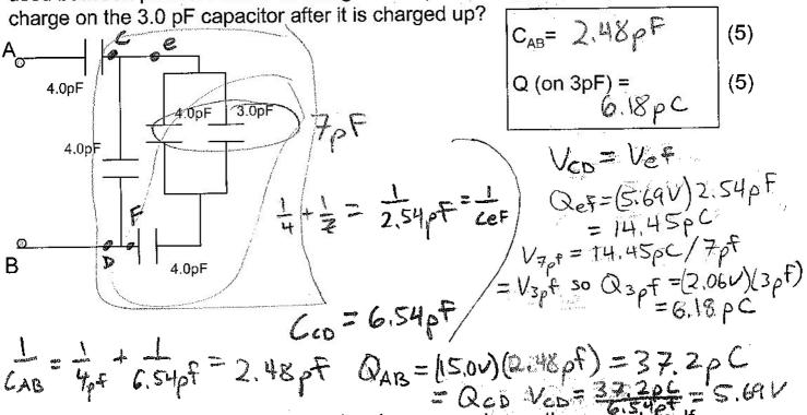
b) Now, the battery is removed, but the charge remains on the capacitors. If an uncharged 2.0 pF capacitor is now hooked up between points A and B, what is the charge on the 3.0 pF capacitor at electrostatic equilibrium?
