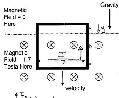
Since the loop is moving at a constant velocity, there must be an equal force acting to hold the loop up. What current do you need to flow in the loop to produce this force? (5 pts) Please indicate the direction of this current on the figure as well. (3 pts) (Hint: find EMF 1st)
