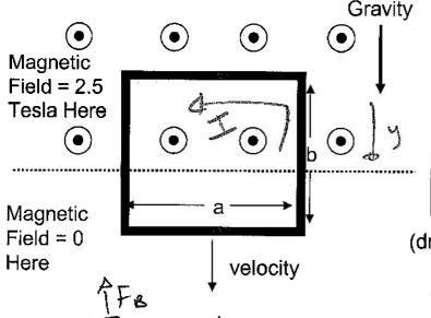
Since the loop is moving at a constant velocity, there must be an equal force acting to hold the loop up. What current do you need to flow in the loop to produce this force? (5 pts) Please indicate the direction of this current on the figure as well. (3 pts) (Hint: find EMF 1st)
