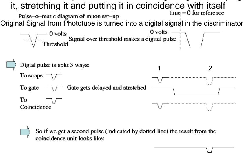
The pulse labeled "1" acts like the first counter, the pulse labeled "2" acts like the second counter, and the total width is essentially the stretched width.
