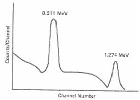
Therefore, the brightest trace you see on the scope when the <sup>22</sup>Na source is place near the scintillator end of the PMT assembly is the 511 keV signal. You may also notice a trace with a peak voltage about 2-3 times larger than the 511 keV signal, but occurring less frequently. That peak is the 1274 keV peak. You should adjust the amplifier knobs so the 511 keV peak is about 2V. You will need to repeat this procedure for both PMT signals coming from the spectroscopy amplifiers.
