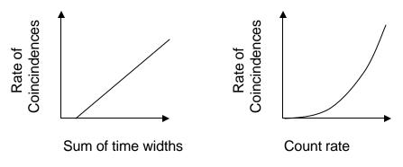
The "count rate" is any time we got a signal above threshold in the discriminator.
