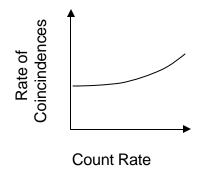
Mathematically, the "Rate of Coincidences" = Rate of Muons that decayed + Accidental Rate
