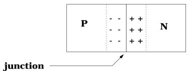
Some of the - charge moves into the P type, and some of the + charge moves into the N type. This happens until there is enough potential difference at the junction of the 2 types of silicon to stop the flow.
