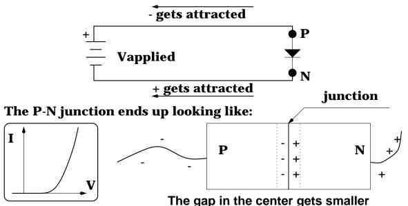
If the voltage is big enough, the gap gets small enough so that charge flows freely. For the diodes you've used in lab before, this is about 0.6 Volts.
