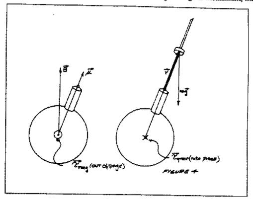
will rotate if the gravitational torque is larger than the magnetic torque, or vice versa. But when the magnetic torque is equal to the gravitational torque, the ball will not rotate, since the net torque on the ball is zero. This configuration is mathematically represented by:
