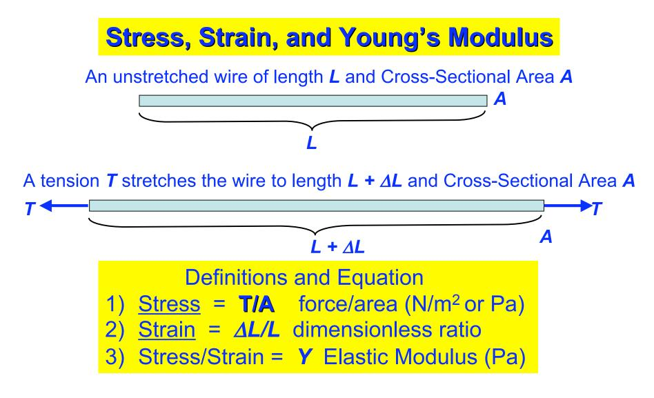
Example: A steel rod has a Young's modulus of 20 x  $10^{10}$  Pa (1 Pascal = 1 N/m<sup>2</sup>) The rod has a cross sectional area of 0.30 cm<sup>2</sup> and an unstretched length 2.0 m The rod supports a weight of 550 kg. How much will it stretch? (T/A)/( $\Delta$ L/L) = Y  $\longrightarrow \Delta$ L = (T/A)\*L/Y = (550\*9.8/(3.0x10<sup>-5</sup>))\*2.0/20x10<sup>10</sup>  $\Delta$ L = 1.8 x 10<sup>-3</sup> meters
